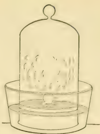
Fig. 56. — Preparation of nitrogen by burning phosphorus in confined air
