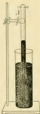
Fig. 50. — Apparatus for determining the volumetric composition of water
