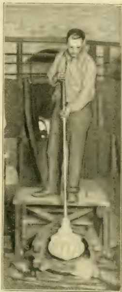
Fig. 144. — The last stage (opening the mold) in blowing an electric light bowl
