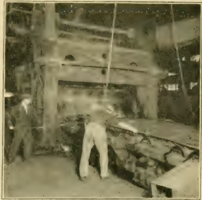
Fig. 185. — Steel plate passing through the last rolling machine
