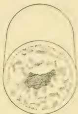
Fig. 169. — Section of a boiler tube showing the scale deposited by hard water
