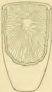
Fig. 92. — Section of a crucible showing monoclinic crystals of sulphur
