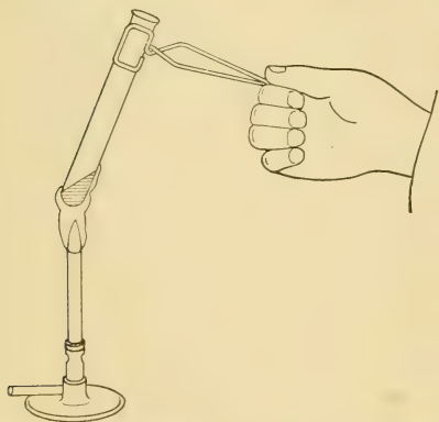
Fig. 2. — Heating a mixture of iron and sulphur in a test tube
