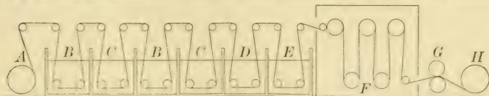
Fig. 64. — Diagram of the process of bleaching cotton cloth
