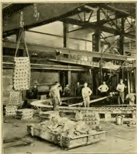
Fig. 207. — Casting refined lead into molds
