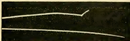
Fig. 218. — Paths of alpha particles (charged helium atoms) in moist air
